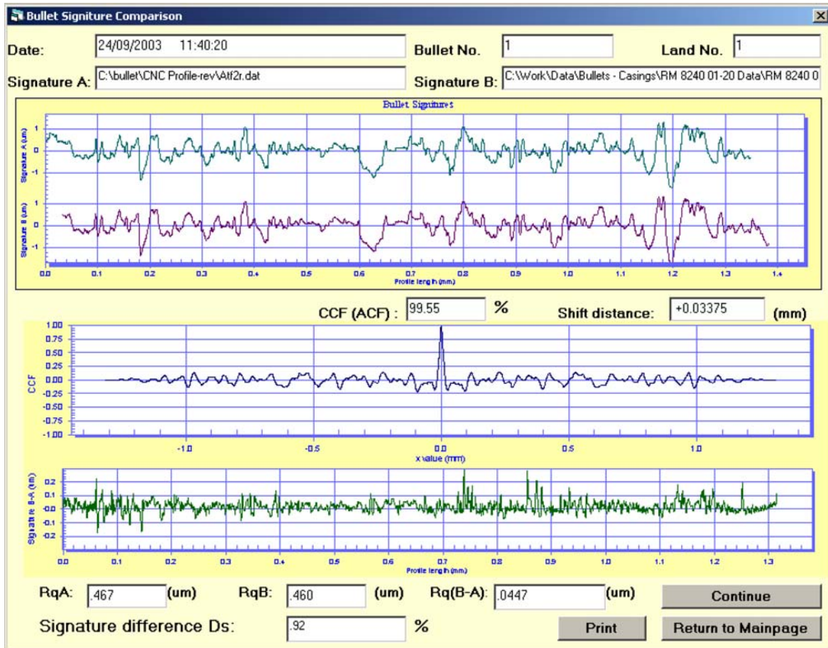
FIG. 6—Bullet signature comparison between the land 1 of S/N RM 8240 001 standard bullet (Signature B, as shown on second profile from top) and virtual standard (Signature A, as shown on top). Cross-correlation function CCF = 99.55\% ; signature difference D_s = 0.92\% .
