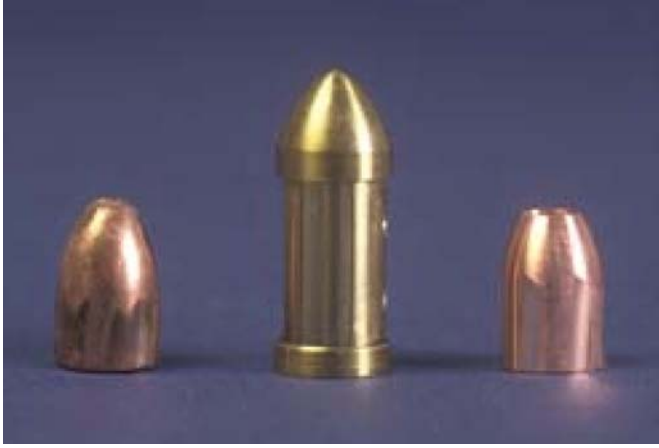
FIG. 1—Master bullet from ATF National Laboratory Center (left), NIST prototype standard bullet (center), and NIST RM 8240 standard bullet (right).
