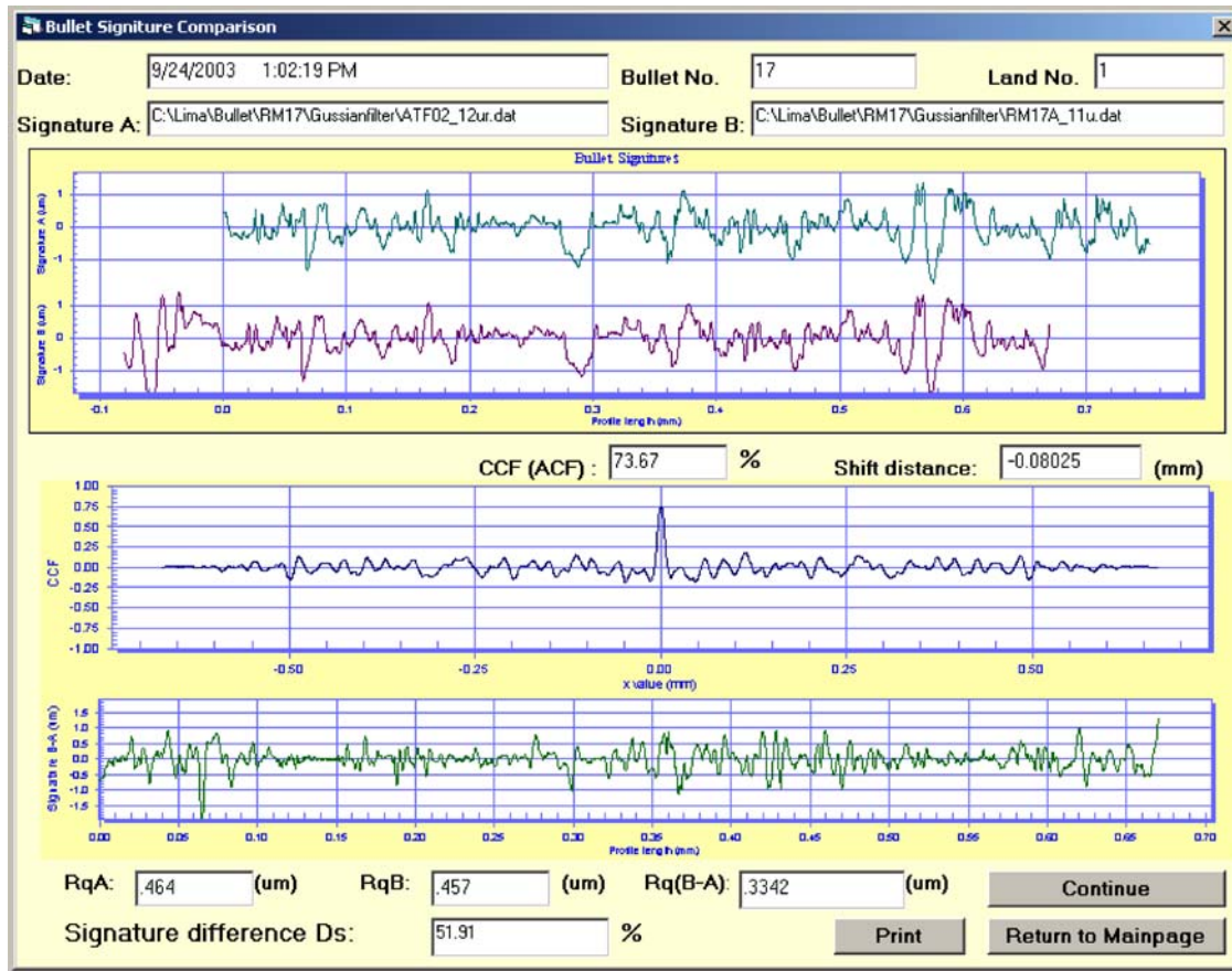
FIG. 8—Bullet signature comparison before the X-scale correction for Signature B: CCF = 73.67%, D_s = 51.91\% .
